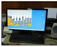
The SCADA system monitors all storage tanks to help ensure constant water pressure and availability.
